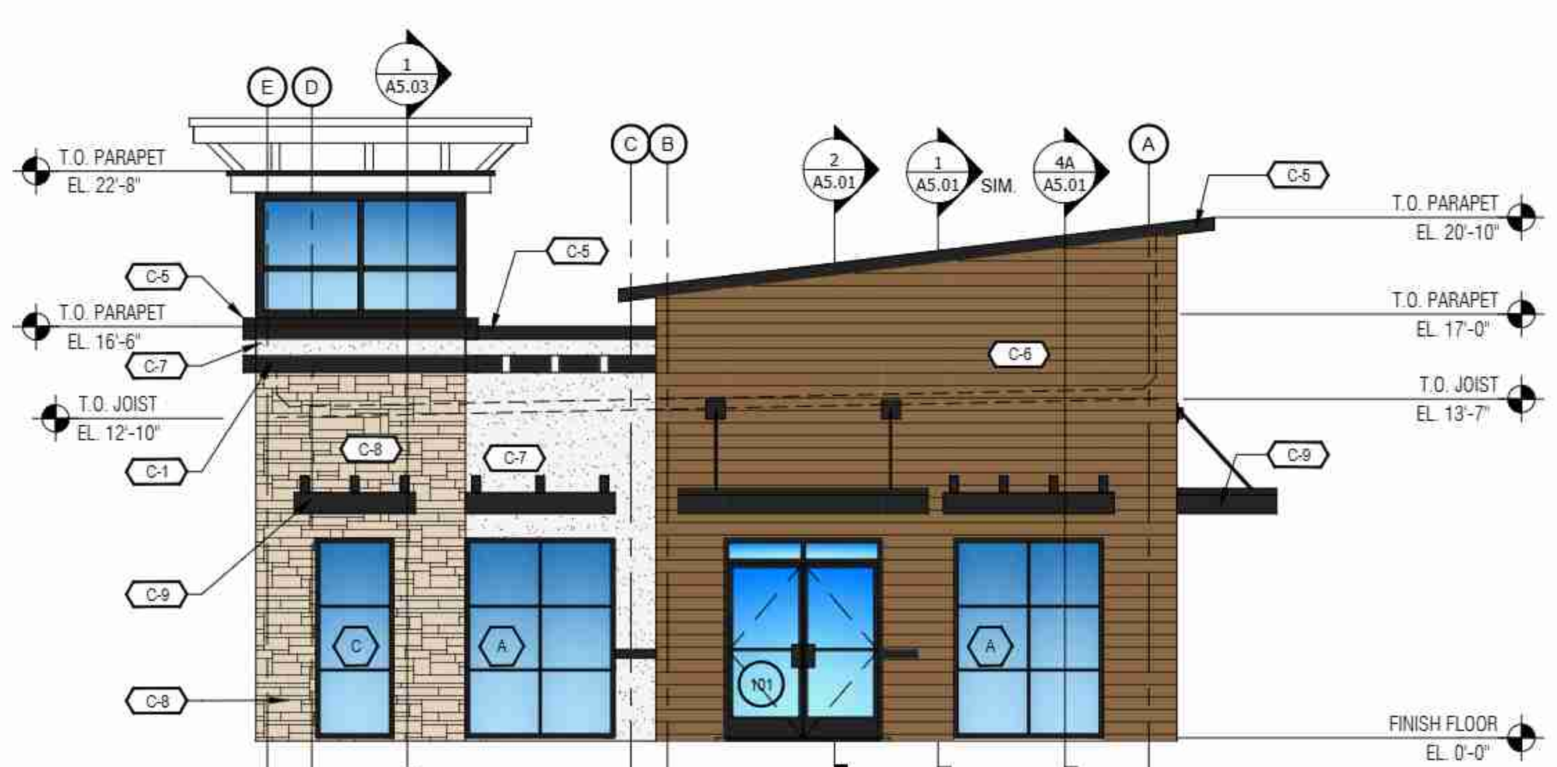
03 EAST EXTERIOR ELEVATION A2.01 SCALE 3/16" = 1'-0" TOTAL ELEVATION (MINUS DOORS/WINDOWS) = 510 (100%) 10 S.F. CEMENT BOARD SIDING (2%) 6 S.F. WOOD TRELLIS (1%) 316 S.F. E.I.F.S. (62%) 140 S.F. STONE (28%) 30 S.F. BRICK (6%)
